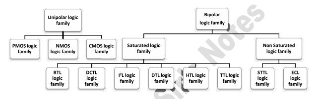
**Unipolar logic families:** The logic circuits in this family contain semiconductor devices, in which current flows due to either holes or electrons. This family contains –
